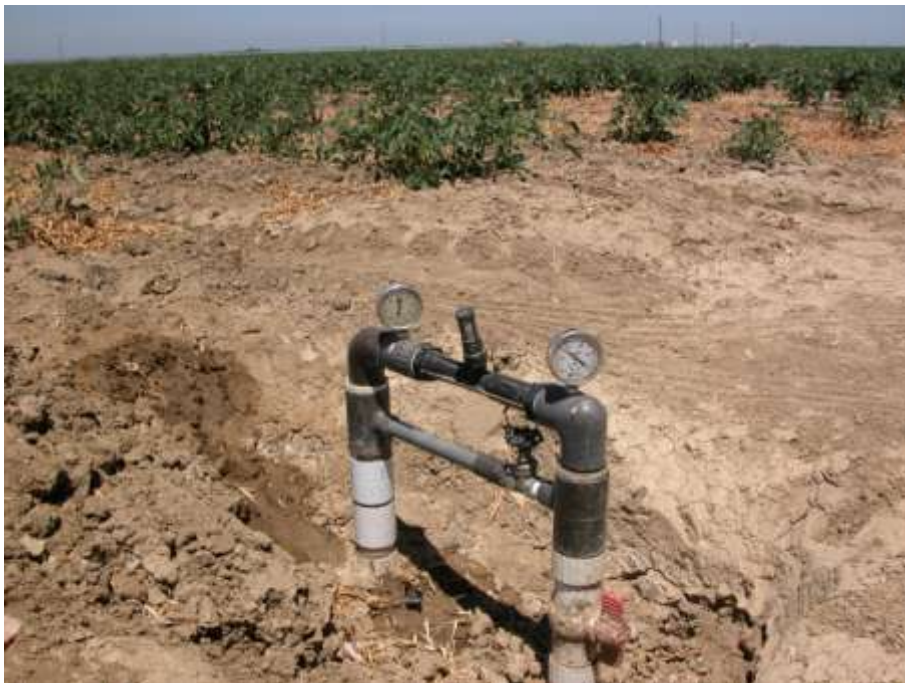
Figure2: Relatively larger injector servicing 24 drip lines.
